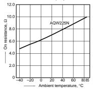
2.-(2) On resistance vs. ambient temperature characteristics
