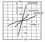
9. Off state leakage current
